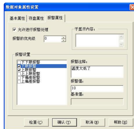
Figure 2-2-9 Setting of Alarm Lower Limit Property
