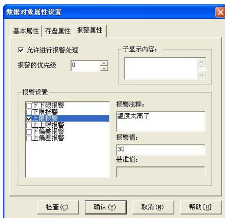
Figure 2-2-8 Setting of Alarm Upper Limit Property
