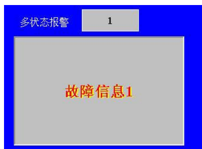
Figure 2-2-16 Operational Effects of Multi-state Alarm
