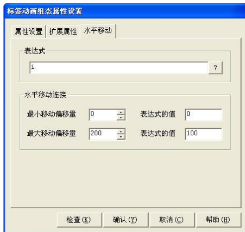
Figure 1-2-4 Property Setting of Horizontal Shift
