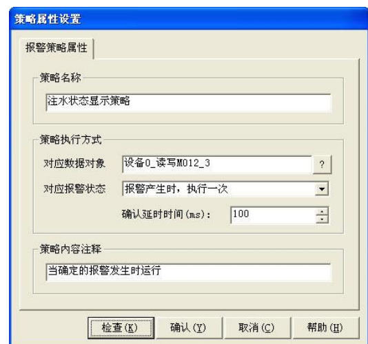
Figure 2-2-19 Property Setting of Level Alarm Strategy
