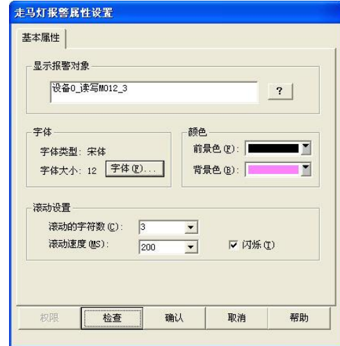
Figure 2-2-5 Property Setting of Alarm Bar
